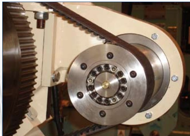
Locking Assembly CfN 7012/CfN 7012-IN · Belt pulley
